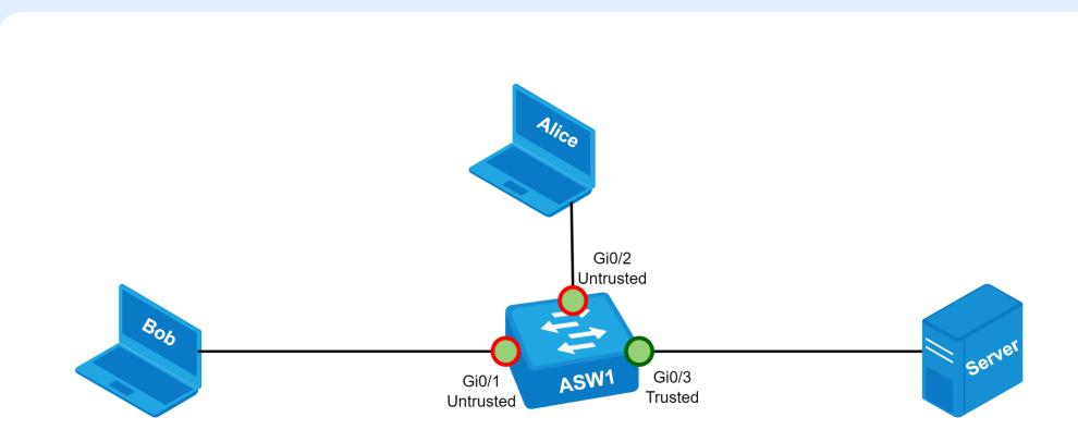
Now that Bob broadcasts the DCHP Discover message, it is allowed at Gi0/1 untrusted port on the ingress, but gets rejected on the egress of Gi0/2 untrusted port.
