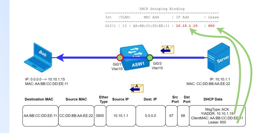
To configure the DHCP Snooping feature at MES 23xx/33xx/35xx/5324 switches according to our example, use the following commands:
