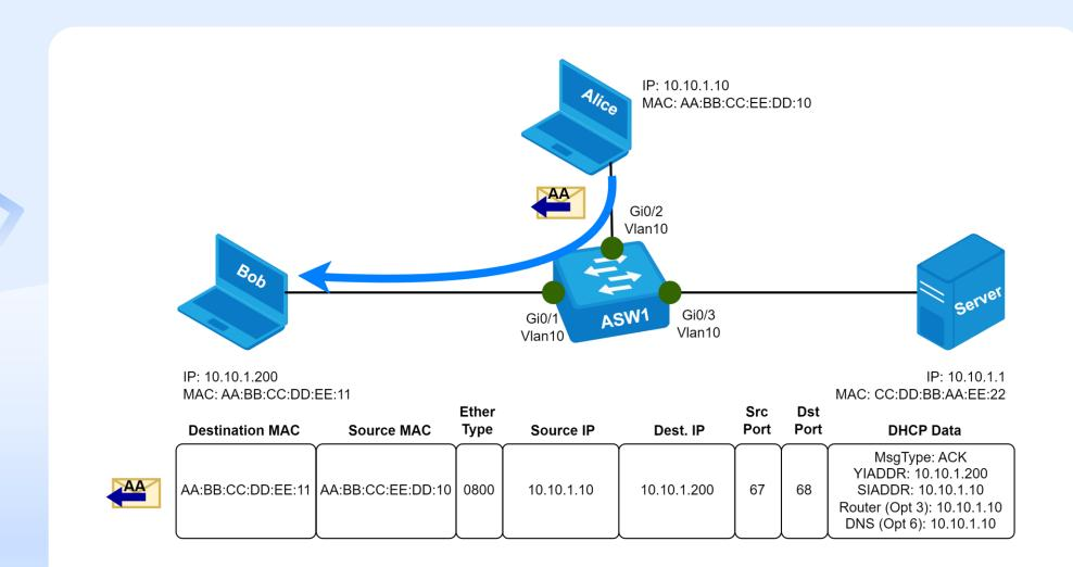
DHCP Snooping is a countermeasure to DHCP Spoofing attacks implemented at L2 or L3 access switches.
